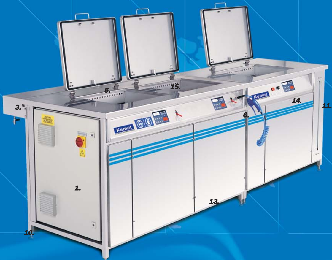
1. Electric box with integrated ultrasonic generator 2. Immersible transducer box on tank wall is protected by robust guide bars. Push-pull rim lip ventilation assisted with compressed air (MC-110) 3. Integrated rim lip ventilation connections behind the tank unit 4. Float switch for dry run protection. All tanks have low level alarms with heating/ultrasonic protection 5. Hinged lid 6. Air gun 7. Tanks are heat and noise insulated 8. Wash basket 9. Internationally recognised, high quality control components 10. Tanks are built within a rigid Stainless Steel framework 11. Sight glass with separate drain valve 12. Stainless drain and water inlet valves at the back of the machine 13. Air bubble agitation in rinse tank 14. Dewatering or hot passivation possible with heating option 15. Profiled overflow weir for optimised surface skimming
